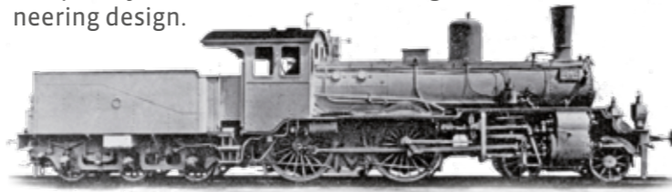
One of the first super-heated steam locomotives using Schmidt'sche Technology built by Henschel Kassel
