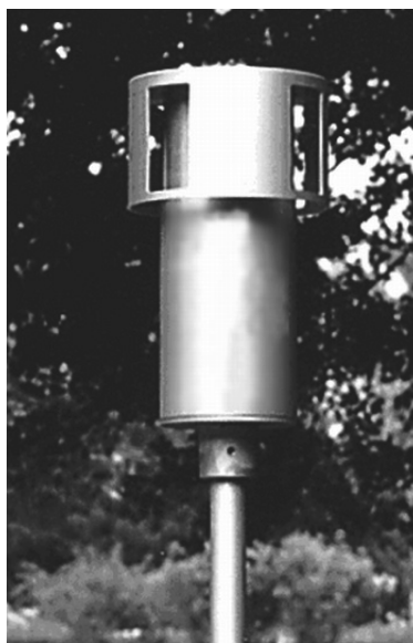
Figure 1. Sigma-2 passive sampler deployed in the field
