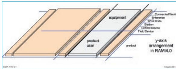
Figure 11. Role-specific arrangement of the assets on the y-axis of the RAMI4.0 architecture
