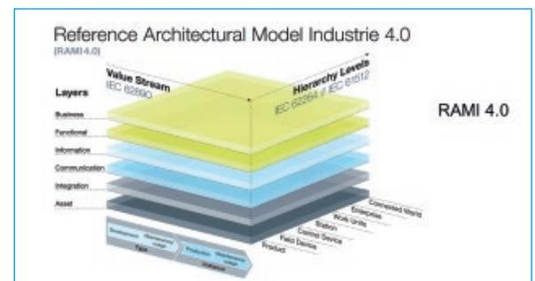
Figure 2. The RAMI4.0 reference architecture [7]
