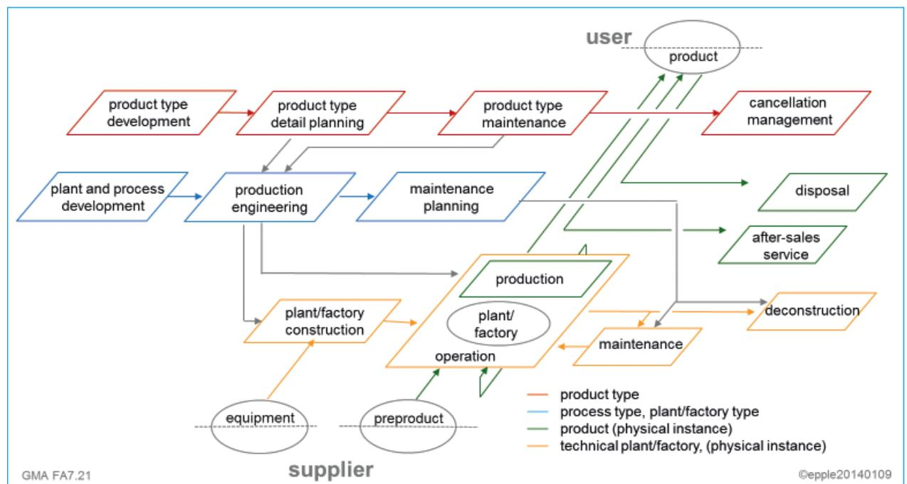
Bild 7. Life-cycle processes - production pattern [11]
